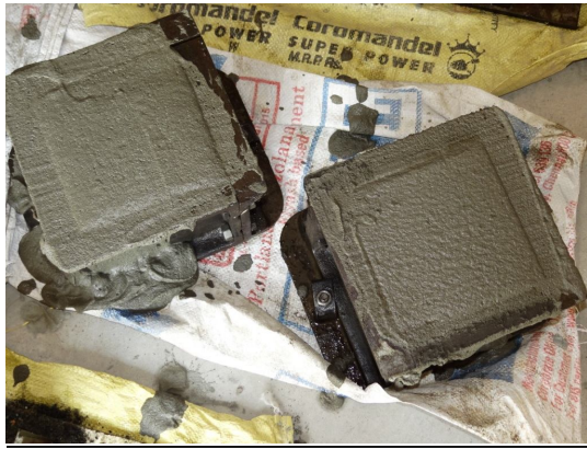
Figure 2. Casting of Cubes
